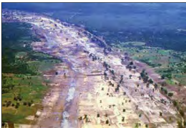
Ingwavuma River outside Ndumu Game Reserve showing massive damage from cyclone Demoina, 1984 (the normal river bed, just a few metres wide, can be seen to the lower right of the photograph)
